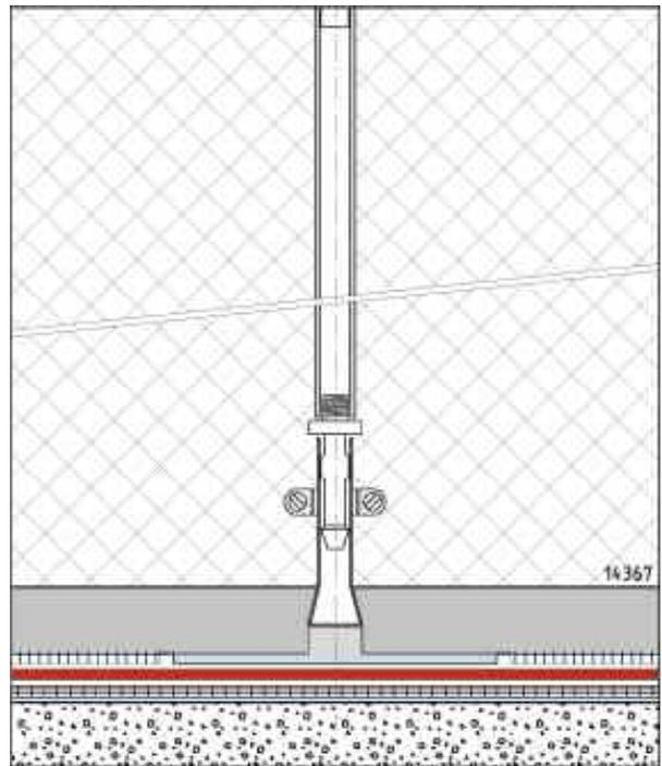
1. Spotwise weld the base of the flange onto the sheet membrane using a heat welding tool.
