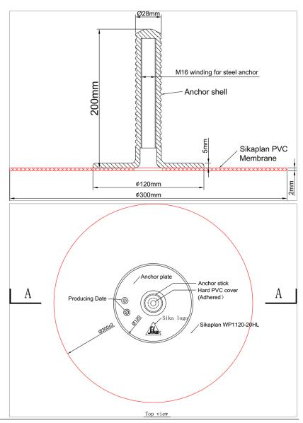
Diameter Shaft: Inside Thread M16, length 200 mm
